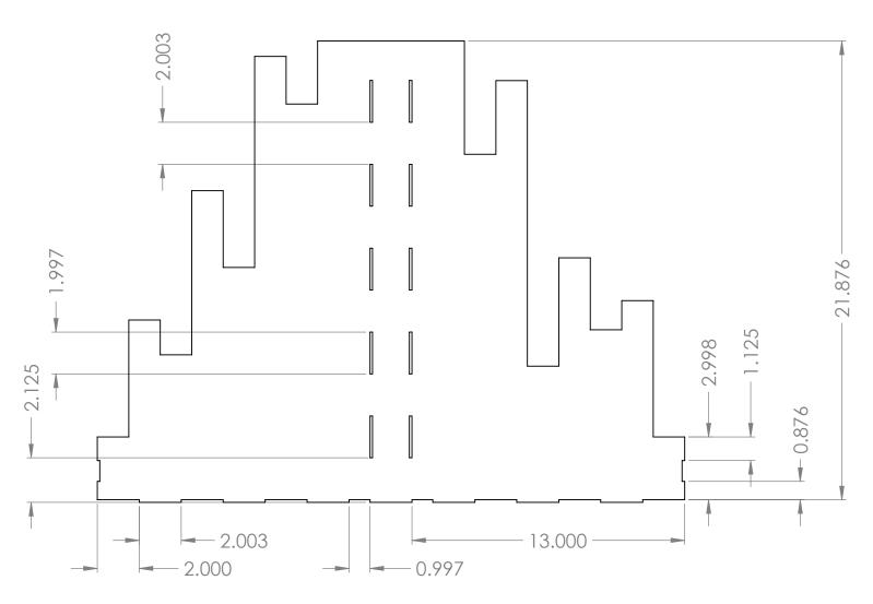
Two-dimensional design to be used on 0.125 inch Duron.
