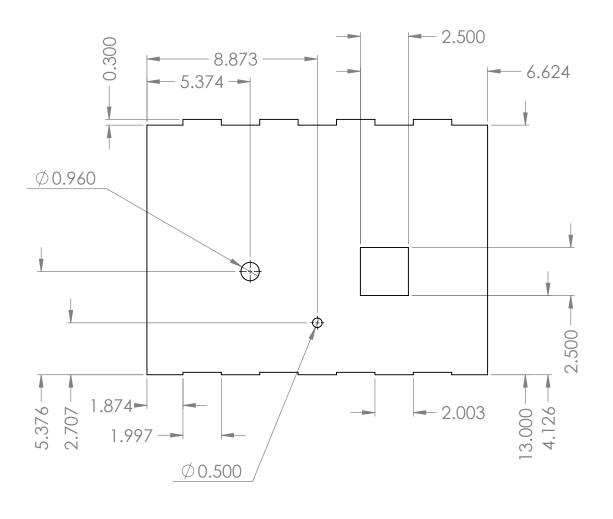
Two-dimensional drawing to be used on 0.125 inch Duron.
