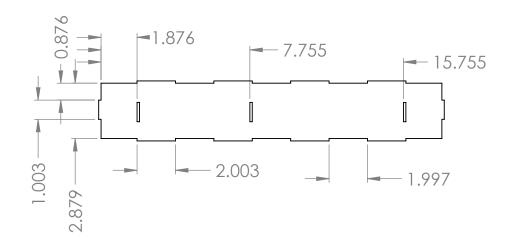
Two-dimensional drawing to be used on 0.125 inch Duron.
