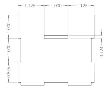
Two-dimensional drawing to be used on 0.125 inch Duron.
