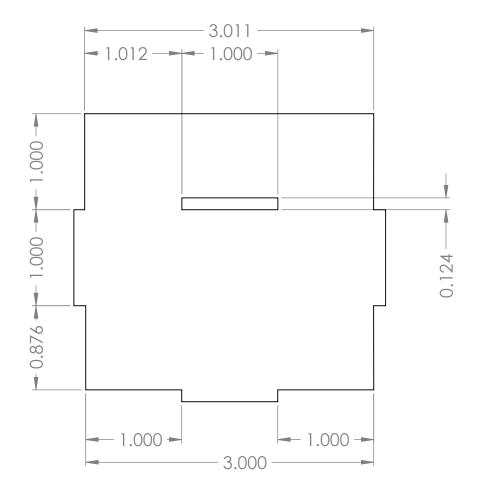
Two-dimensional drawing to be used on 0.125 inch Duron.
