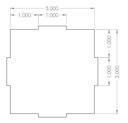
Two-dimensional drawing to be used on 0.125 inch Duron.
