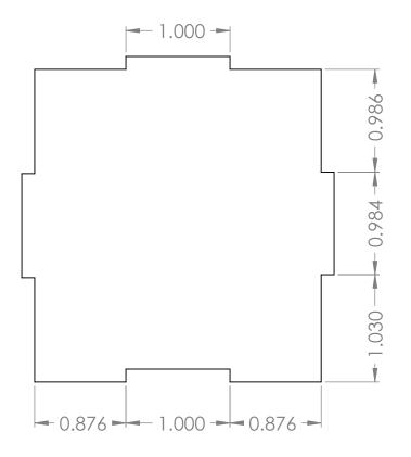
Two-dimensional drawing to be used on 0.125 inch Duron.
