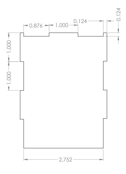
Two-dimensional drawing to be used on 0.125 inch Duron.
