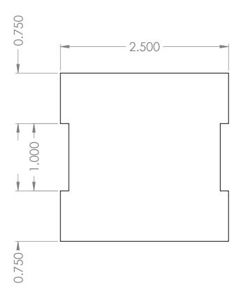
Two-dimensional drawing to be used on 0.125 inch Duron.
