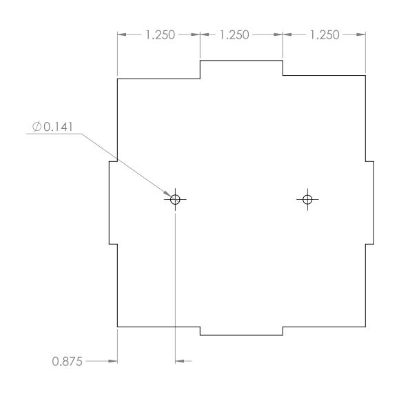
Two-dimensional drawing to be used on 0.125 inch Duron.
