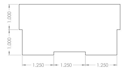
Two-dimensional drawing to be used on 0.125 inch Duron.
